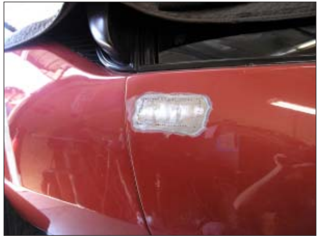
Above: The door handles were removed and panels were crafted to fill in the void by Josh. Below: Front view of the newly formed fenders. Note how body crease flows into the flares.
