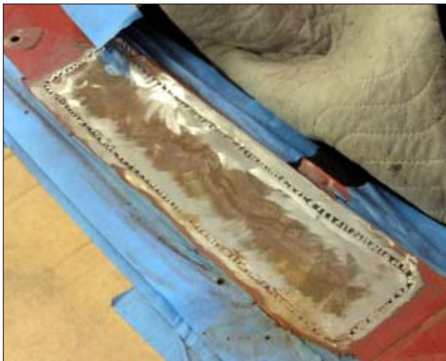
Below: Very few shops in the Pantera industry have the capability to do metal work like this in-house. PI Motorsports, Inc. has a superb metal crafter, Josh Winderman on our staff that can do this precision type work. The fender flares fit the wheels and tires like a glove. Chris preferred using steel over the original fiberglass type the factory used on the real Grp IV.
