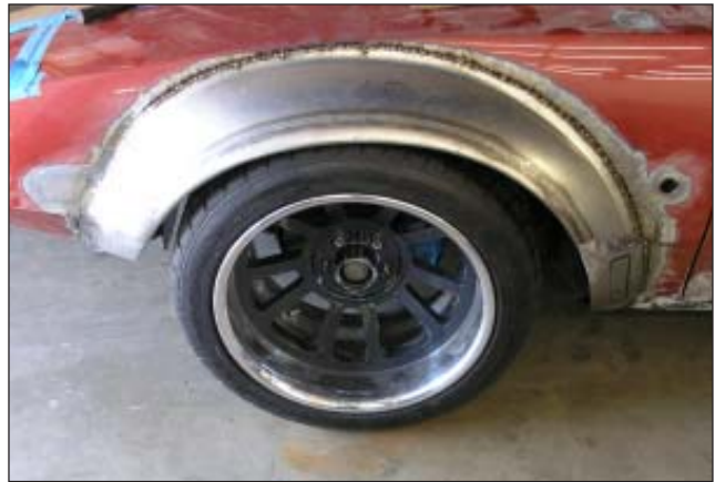
Above: The luscious Grp. IV fender arches are welded into place. Below: The side marker and relief vents have been cut.
