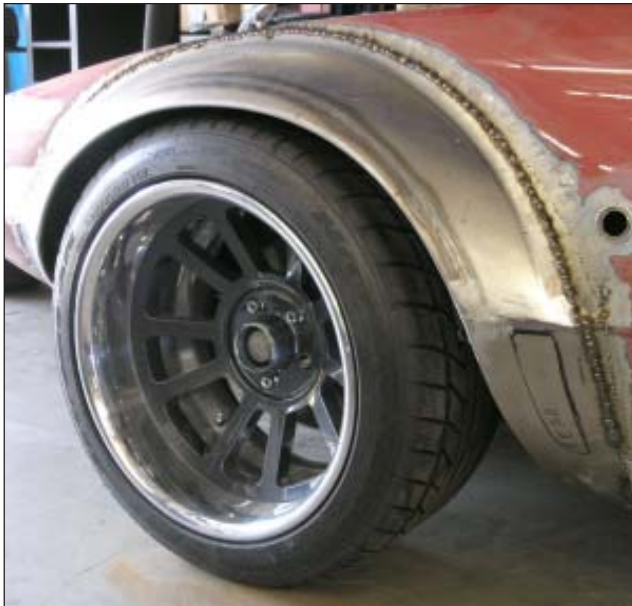
Below: Very few shops in the Pantera industry have the capability to do metal work like this in-house. PI Motorsports, Inc. has a superb metal crafter, Josh Winderman on our staff that can do this precision type work. The fender flares fit the wheels and tires like a glove. Chris preferred using steel over the original fiberglass type the factory used on the real Grp IV.
