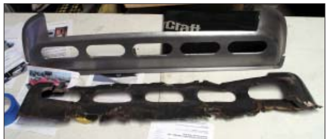
Above: Close-up of the owner designed exhaust vents. Below: The original metal work showed rust and new steel was used in replacement.
