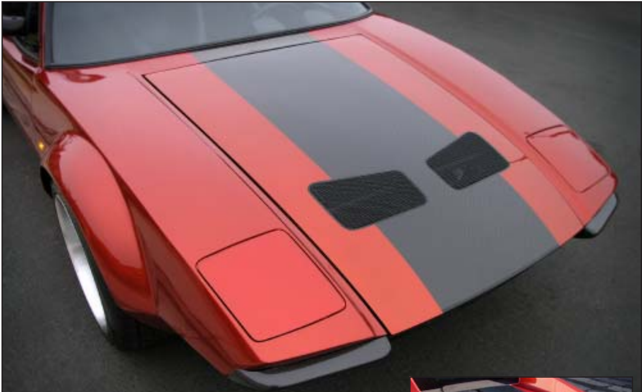
Above: The air vents were custom shaped and fabricated and are a refreshing change from the GT5 type units from DeTomaso.
