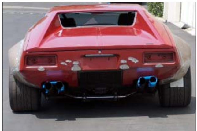
Below: The bumpers were removed and all holes were filled and smoothed.
