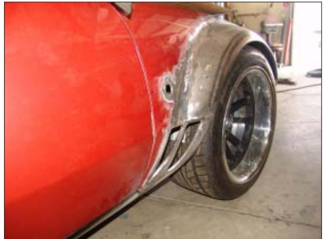
Above: The luscious Grp. IV fender arches are welded into place. Below: The side marker and relief vents have been cut.
