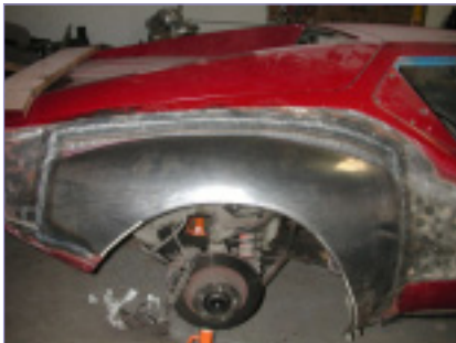
Above and below: The fenders were carefully fitted to the wheels and tires for correct look.
