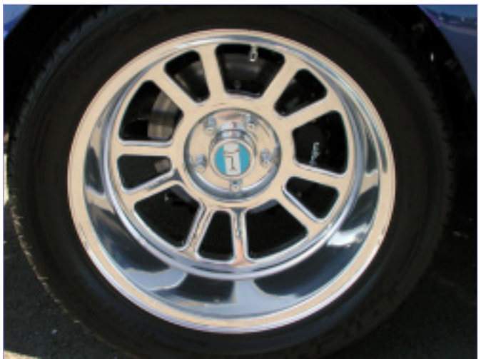
Above: 17-inch diameter rims are 11 inches wide in the rear and 8.5 inches in the front. Michelin rubber meets the road. Disc brakes are from Wilwood.
