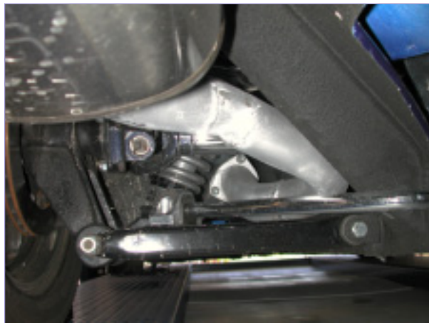
Above: The suspension parts were powder coated in black satin finish. The shock absorbers are aluminum PI Motorsports, Inc. adjustable units. The half shafts are chrome plated.
